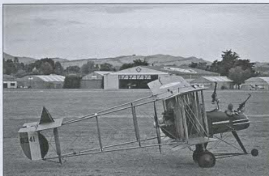
• Fig 4. A reproduction FE2B built by The Vintage Aviator Ltd, Masterton, NZ in 2009. (Courtesy: Phillip Capper, Wellington, NZ).
