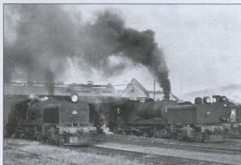
• Garratt locomotives at Nawalapitiya running shed being fired in preparation in going into service. All photos by Les Nixon.
