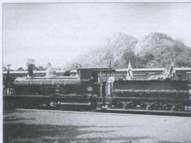
• Figure 1: Class ML 4-4-0 Steam Locomotive - circa 1870.
