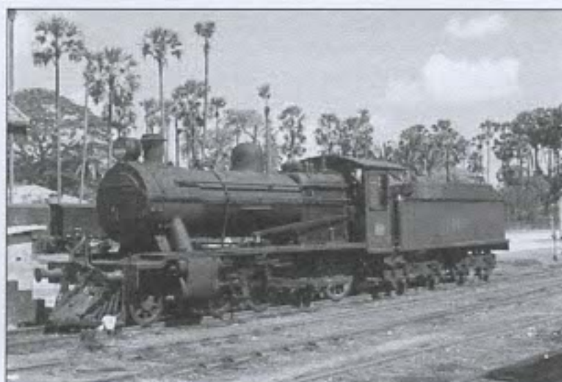
• Figure 3: Class B1 4-6-0 Steam Locomotive.
