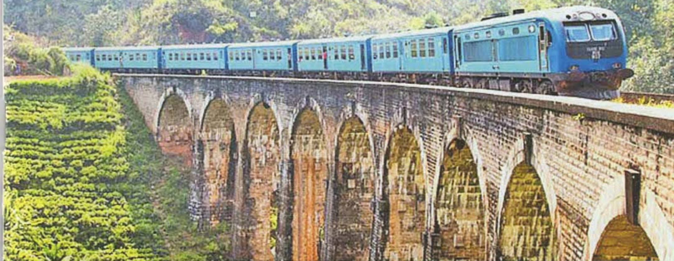
Figure 12 (above): Class S12 2x1,950 hp CSLRSC Diesel Electric DMU running on the nine arch viaduct in Demodara, Sri Lanka
