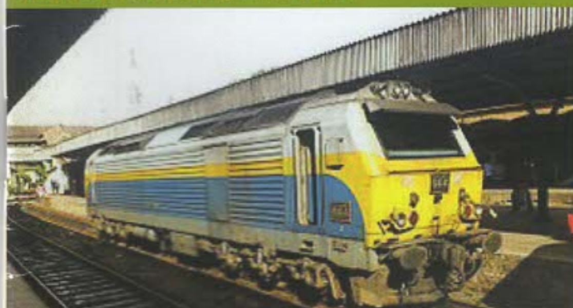
Figure 10: Class M9 Co-Co 2,500 hp Alstom Diesel Electric Locomotive
