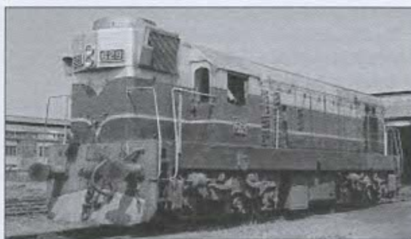
• Figure 9: Class M2 A1A-A1A 1,425 hp GM-EMD Diesel Electric Locomotive.
